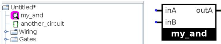
This is the default appearance of a sub-circuit, this can be customized by clicking the “Edit circuit Appearance” button in the Tools/Views pane.
